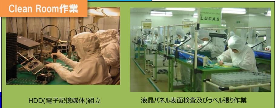
Workers in white cleanroom suits are working in a clean room environment. One worker is assembling an HDD, and another is inspecting a liquid crystal panel.
