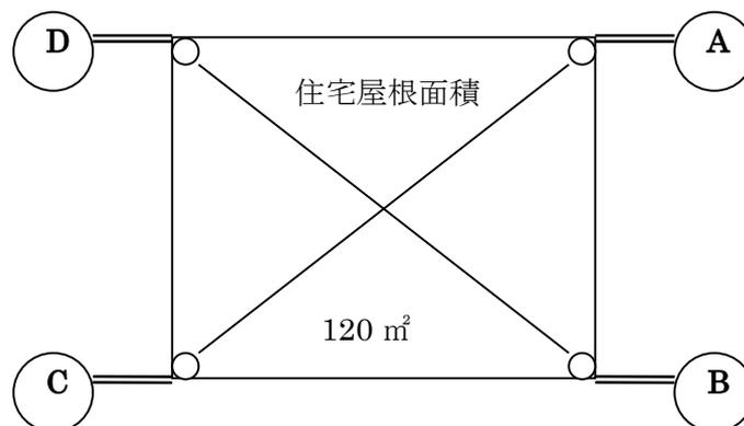
$$A \cdot B \cdot C \cdot D \text{ の浸透ます} = \frac{120\text{m}^2(\text{住宅屋根})}{4} = 30\text{m}^2$$
